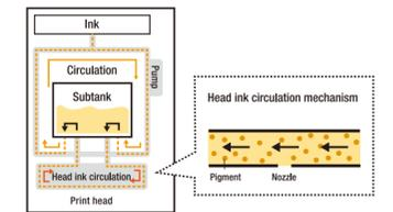
**NCU (Nozzle Check Unit) for automatic self-recovery of clogged nozzles** The world's first<sup>5</sup> 3D printer equipped with an NCU for auto detection of ink misfiring due to clogged nozzles. When a missing droplet is detected, the head moves into auto cleaning for recovery. Detection frequency can be set by time or day, preventing possible modeling errors.
