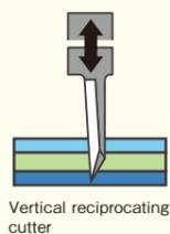
The blade cuts thick materials by a vertical reciprocating motion. It is ideal for foam or cardboard cutting. In addition, the blade is capable of cutting a range of material thicknesses, from thin to thick, by precisely controlling the blade edge direction. (Before cutting, please place a felt mat on the cutting table under the material to hold it in place.)
