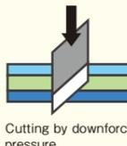
The blade edge is automatically and precisely controlled along contour cutting lines specified by the software. It is good for cardboard and foam board.
