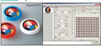
Total printing time (White printing+Color printing): 22 min., 24 sec. Size: 29 mm dia., 1200 × 1200 dpi, 16 pass Hi-mode Width 600 mm x feeding direction 500 mm, with 168 units imposed.
