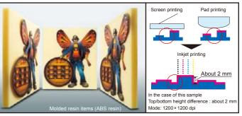
Note: To prevent the occurrence of problems due to ink mist when printing on three-dimensional items, the area around the head should be cleaned frequently. Also, the greater the distance from the head, the more the printing quality declines, so prior testing is necessary.
