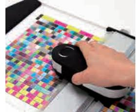
Color measurement with a colorimeter
