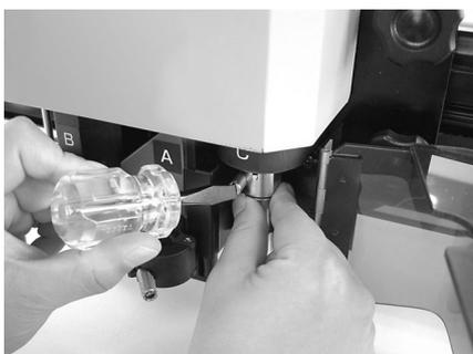
**Tighten the stopper screw with the screwdriver supplied with the device as an accessory.**
