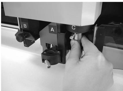
**Insert the pin of unit C into the marking roller while fitting the pin in the groove on the roller.**
