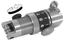
**Tighten the cutter stopper.**
