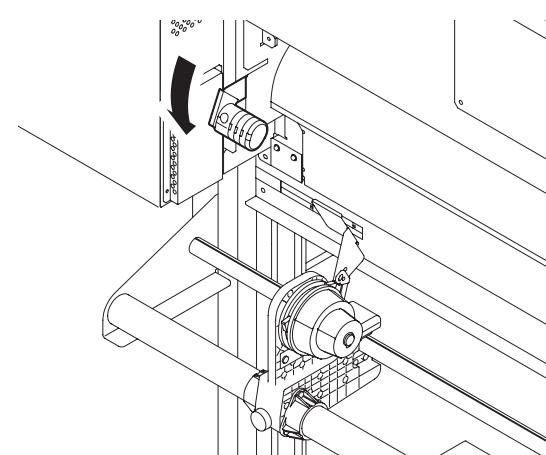
(3) Move the roll holder to the roll setting position.
