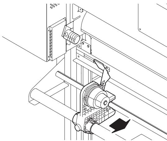
(2) Check the clamp lever is lowered.
