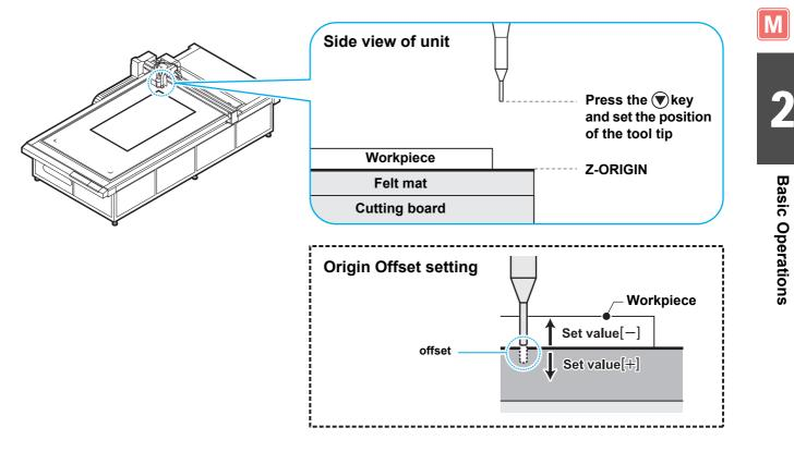
• Always reset the Z-axis origin after changing the head height. Using the unit without resetting the Z-axis origin can damage the unit, if the end mill is pushed through the cutting panel, for example.
