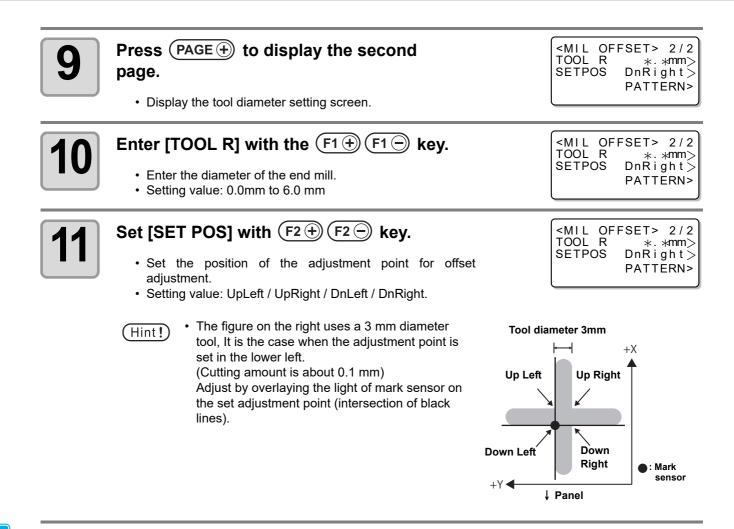
If you want to write a new adjustment pattern, move the head with the jog key and press ( $F3 \oplus$ ).
