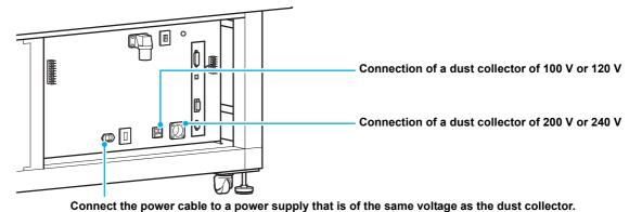
• The voltage from the power cable for dust collection cannot be automatically converted and output to the voltage of the connected dust collector. Be certain to connect a dust collector that matches the power
