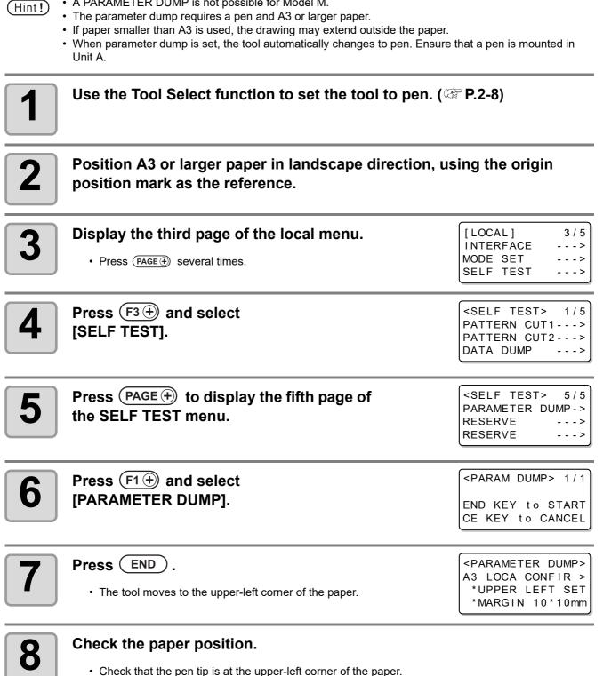
• If the pen tip is not located at the upper-left corner of the paper, align the upper-left corner of the paper with the pen.
