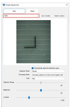
**5** Adjust the settings below while checking the image captured until the register mark is correctly enclosed within the red frame. <sup>(2)</sup> "[Detect Setting] Screen Layout"(P. 18)
