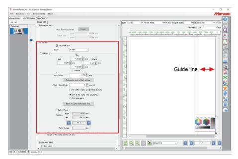
7 Select the slitting method for the Y (scan) direction.
