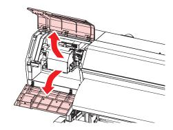
**?** Remove the side screw, and detach the media holder stopper.
