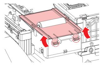
5 Remove the cloth wiper together with the spindle, then replace it.
