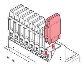
**?** Remove the ink absorber, and replace with a new one.
