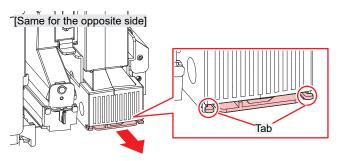
5 If the glass holder is also replaced together, cut the tabs on the rear side.
