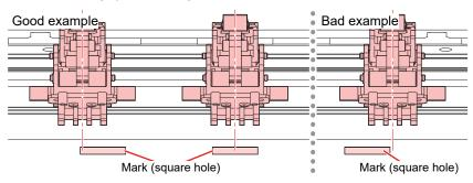
Mortant! Alter the XY clamp positions according to the RasterLink [Y Slit] setting.
