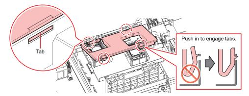
7 Remove the maintenance liquid absorber.
