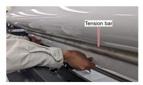
6 Insert the media between the pinch rollers and the grit rollers of the XY slitter.
