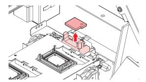
**7** Wipe away any maintenance liquid from around the slider block.
