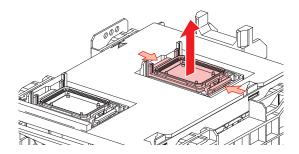
[When using Sb ink and TP ink] Rinse the cap with the mesh side facing downward in a container filled with maintenance liquid. Remove, then wipe clean the resin part thoroughly.
