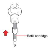
3 Insert the spring into the refill cartridge.
