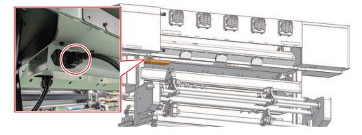
**?** Check to confirm that the power plug is connected to the power outlet.
