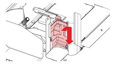
Attach the cap to the removed waste ink tank, and use tape to prevent leakage of waste ink.
