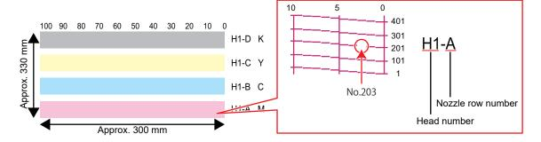
▲ Select the "head number and nozzle row" for nozzle recovery, then press the [ENTER] key.
