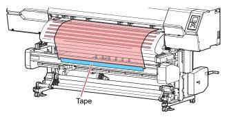
(2) Pull the media toward the take-up unit while spreading it out slightly evenly on both sides to prevent sagging.
