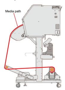
For details of how to load roll media, refer to "Loading the Roll Media" (P. 78).
