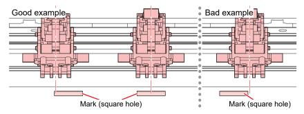
Module: Alter the XY clamp positions according to the RasterLink [Y Slit] setting.
