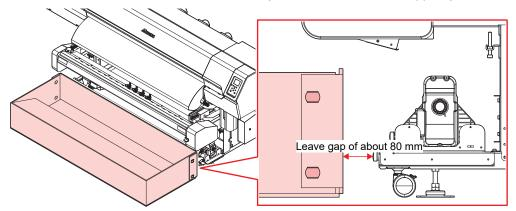
If the prints make contact with the media chute, move the media chute closer to the machine.
