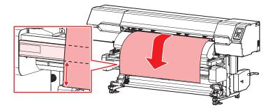
5 Engage the media on to the tension bar and pull it out from the bottom.
