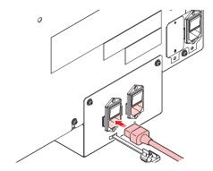
**?** Check to confirm that the power plug is connected to the power outlet.
