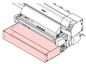
• Pattern 2: If problems occur when arranged as described above, turn the media chute around so that the front is at the rear. (Do not use the media support.)
