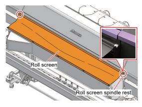
When not in use, the roll screen can be rolled up and stowed at the front.
