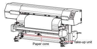
2 With the clamp lever raised, perform steps (1) to (4) below to secure the media to the paper core.
