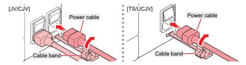
5 Plug the power plug into the power outlet.
