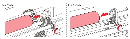
Insert the media between the pinch rollers and the grit rollers.
