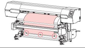
10 Press To wrap the media about one and a half turns around the paper core, then press the [ENTER] key.
