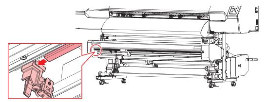
**7** Turn the screw and remove the cutter.
