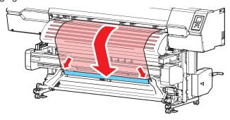
(3) Attach the media to the take-up unit, ensuring an even tension on both sides.
