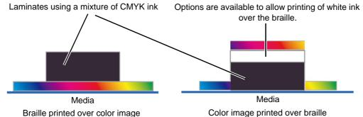
•A mixture of CMYK ink is laminated to the specified height for the braille.
