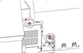
(2) Pull the cover in the direction of the arrow to remove the mist filter.
