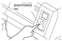
• The firmware version is displayed when the power is turned ON, and then the machine performs its initial operation.
