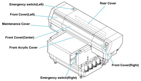
\*7151plus has no interlock for front cover (center) and rear cover.
