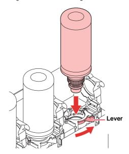
8 Move the lever on the tank completely from the right to the left side.
