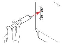
Made mixed water (antifreeze liquid: 1, water: 2) in the attached reservoir and move it to the attached syringe.
