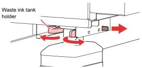
**(2)** Pull it frontward to remove by holding the waste ink tank handle.
