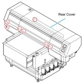
\*7151plus has no interlock for front cover (center) and rear cover.
