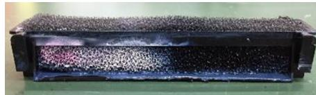
**6 Reinstall the mist filter in its original position.****7 Once cleaning is complete, close the cover, then press the [ENTER] key.****Blowing Fan Filter Cleaning**
