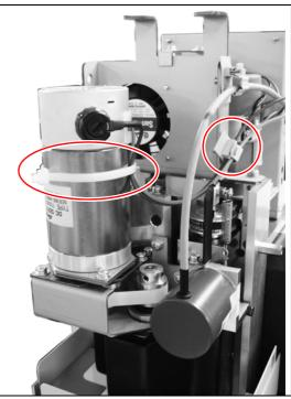
**5** Remove the CN7 connector from the PCB.
