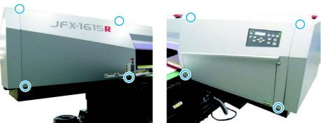
• The cooling fans are on the circled places (6 places) shown on the below. When replacing the cooling fan filter, replace all the filters.
