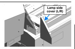
**9** Remove the socket cover of both sides of the lamp.
