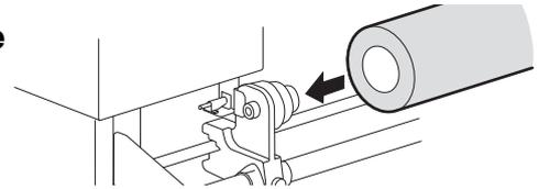
**6 Loosen the screw of the right side roll holder then insert the holder into the core of the roll media.**
