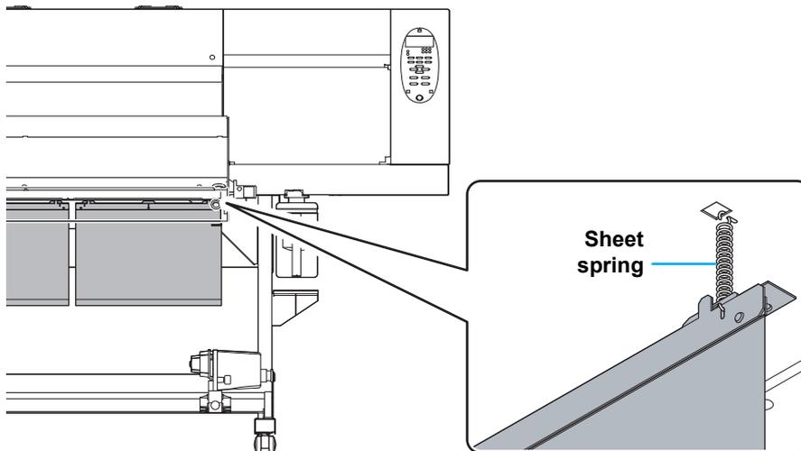
If you removed the antistatic sheet, attach the sheet holder on the platen (130LX: three positions / 160LX:four positions).
