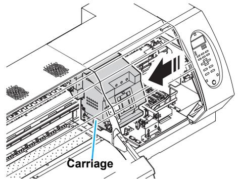
**5** Open the right maintenance cover cover then remove the wiper.
