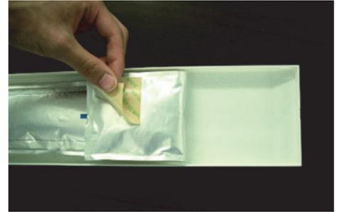
**3** Firmly fix the ink pack on the eco case with double coated tape so that it may not move.
