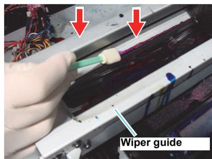
**Wiper guide upper portions and portions one level below****12****Press the **ENTER** key after the cleaning.**
