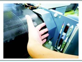
Be sure to insert a stopper if working around the pressure roller.
